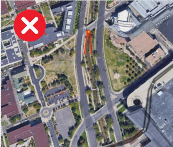
Bad Location: Narrow river is below ground height with trees and tall buildings.
