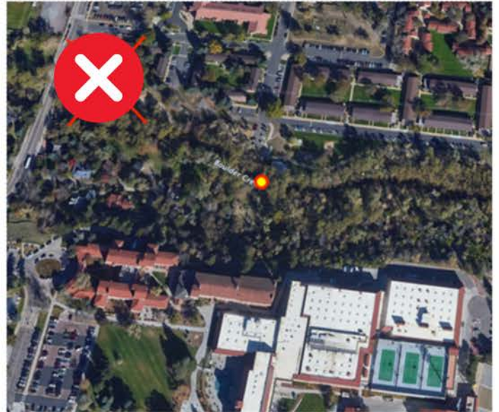
Bad Location: Narrow field of view with obstruction from thick tree cover and buildings.
