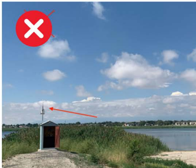
Bad Installation: Obstructions in the field of view of the water.
