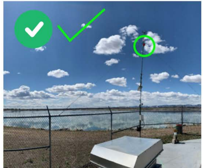
Good Location: Southern field of view to the water with no obstruction.
